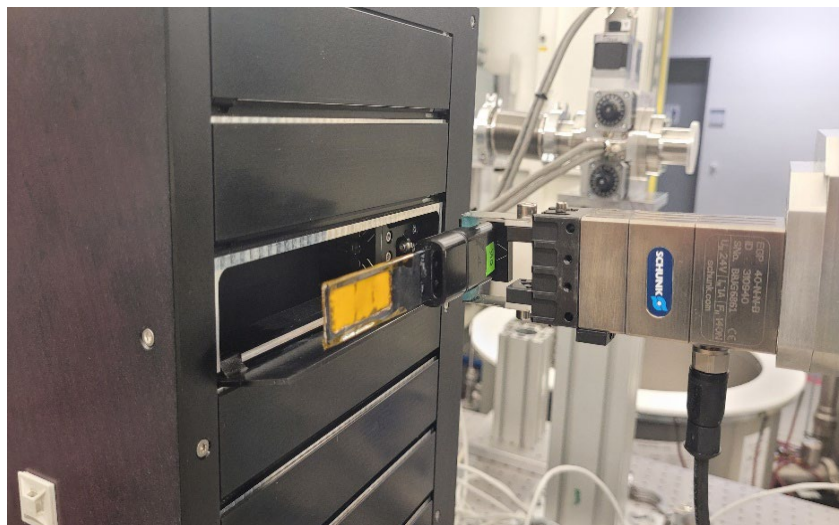
Figure 4: Gripper tool moving sample from the room temperature storage container
